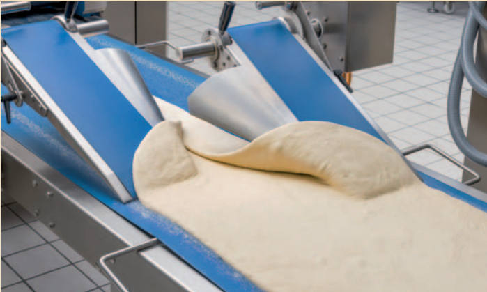
Folding the bread dough increases stability and volume of the rolls.
