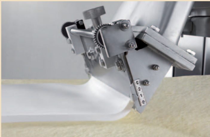
The special engineering design means that the fat pump only has a marginal influence on the temperature of the fat.
