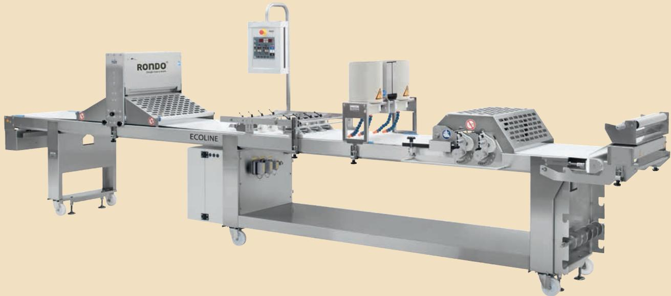
The Ecoline is a compact make-up line which allows you to begin automated production for folded and rolled pastry products. Designed and manufactured in our factory in Switzerland, it unites all the qualities that characterise RONDO machines at a low price.
