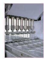
Standard nozzle: 1 needle by output
